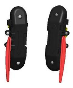
Replacement/Repair components for Thomas Built Bus Window assemblies.
