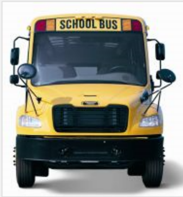
Foreground - Hawkeye® front cross view mirror assembly. Background - DuoStyle® assembly w/black arms
